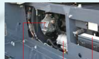
Generator Starter motor Fuel box
