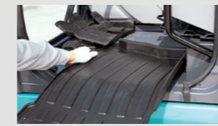
Detachable two-piece floor mat has handles for easy removal. A floor drain is located under the mat.
