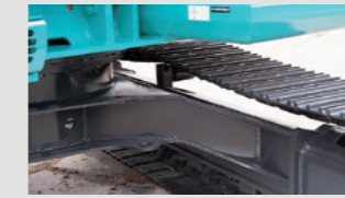
Special crawler frame design makes it easy to clean off mud.
