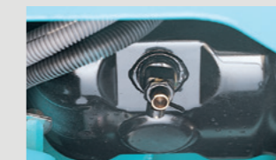
Engine quick-drain valve can be turned without tools.
