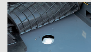
Washer fluid tank is located under the cab floor mat.
