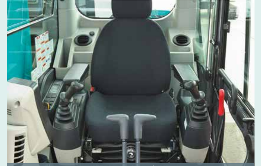
Seat suspension absorbs vibration
