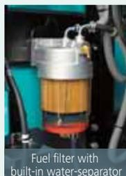
Fuel filter with built-in water-separator
