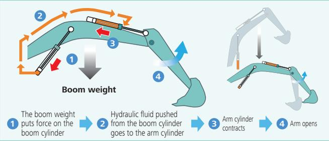
**Hydraulic circuit reduces energy loss**
