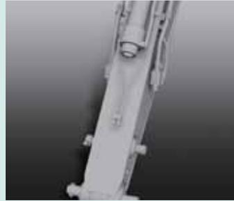
A quick hitch hydraulic line, which speeds up attachment changes, is available as a standard.
