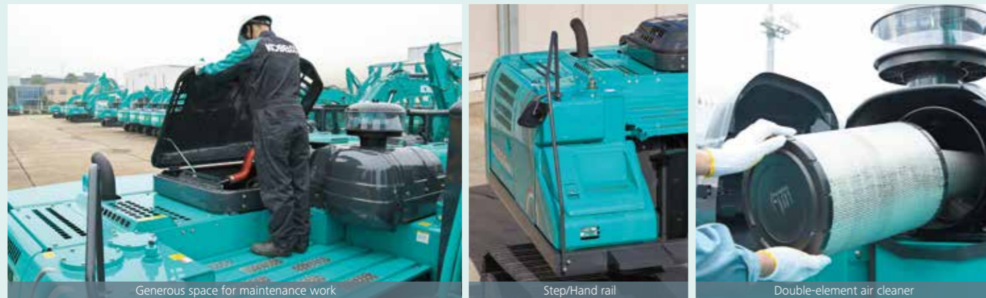
Generous space for maintenance work
