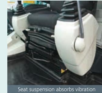
Seat suspension absorbs vibration
