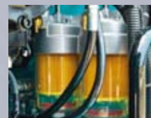
Pre-fuel filter (built-in water separator) The large capacity fuel filter is designed specially for common rail engines. This high-grade filter catches 95% of all dust particles and other impurities in the fuel.
