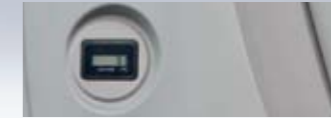
Hour meter Hour meter can be checked while standing on the ground.
