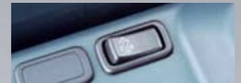
DPF reactivation switch If the monitor warning goes off, the filter should be reactivated manually using a switch.
