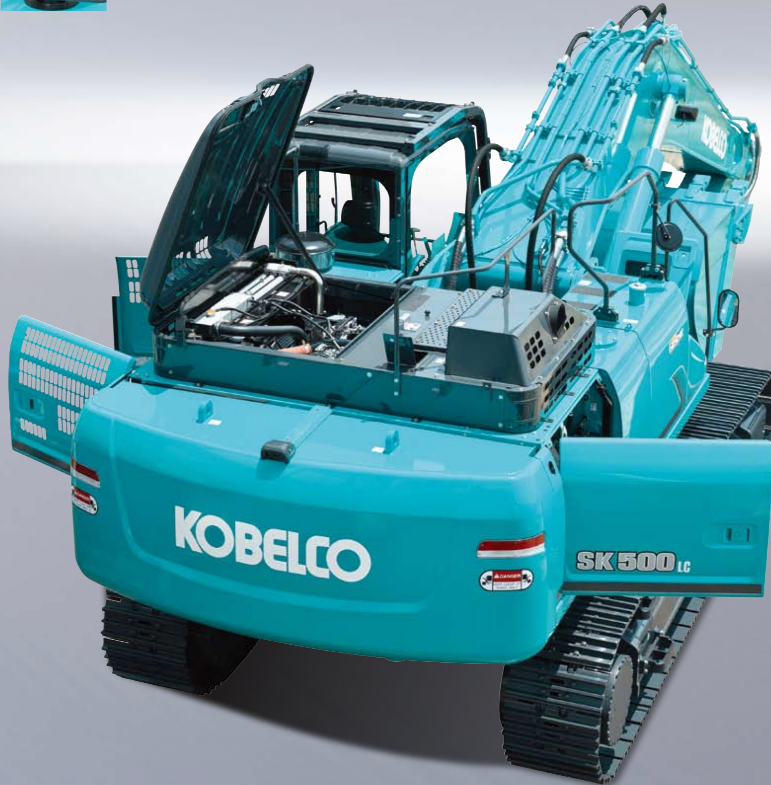
Double-element air cleaner The large-capacity element features a double-filter structure that keeps the engine running clean even in dusty environments.
