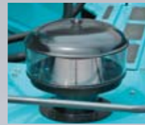
Pre-air cleaner The pre-air cleaner prolongs a replacement cycle of main air cleaner.
